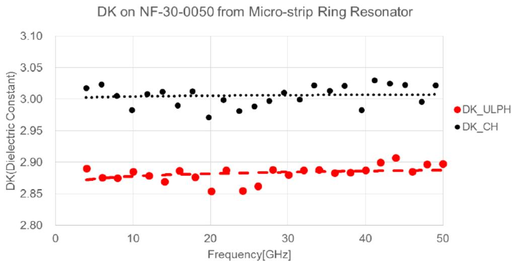
NF-30 is supplied with ULP copper foil, an Ultra-Low Profile copper foil due to its superior insertion loss at 77 GHz. The slightly lower Design DK is easily adjusted in any CAD program.
