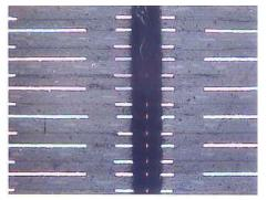
Figure 2 - Multilayer containing TSM-DS3 and fastRise27
