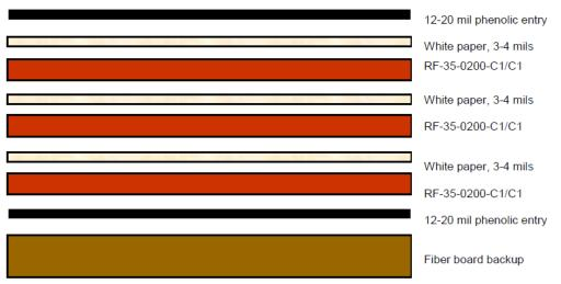
Figure 7 – Typical TSM-DS3 rout stack-up
