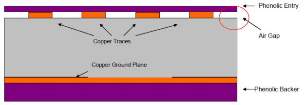
Figure 6 – A typical rout stack with phenolic entry and backer material on either side of the circuit board
