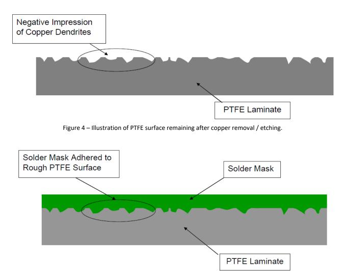
Figure 5 – Illustration of soldermask wetting and adhesion to rough PTFE surface.
