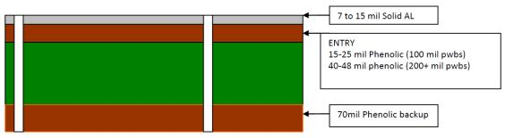
Figure 3 – Stackup of Multilayer Drilling
