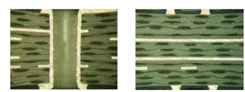
Microsection of 6 copper layer multilayer containing RF-60TC-0100 and *fast*Rise™7 prepreg (PWBs courtesy of Delta Circuits, Fairfield, NJ)
