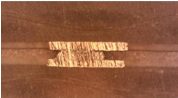
fastRise TM prepreg between subassemblies w/copper paste
