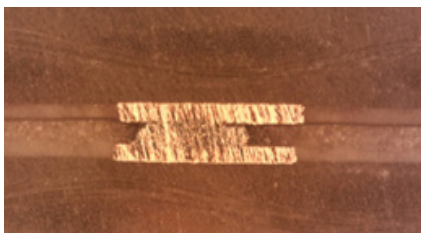
fastRise TM prepreg between subassemblies w/copper paste
