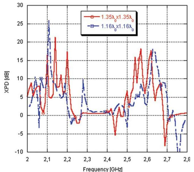
**Figure 9** Comparison between the XPD of the antenna backed by the  $6 \times 6$  sized screen (straight line) and the  $4 \times 4$  sized screen (dashed line). [Color figure can be viewed in the online issue, which is available at [www.interscience.wiley.com](http://www.interscience.wiley.com)]
