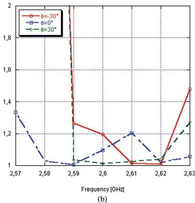
**Figure 4** (a) Axial ratio of the spiral closed to the AMC screen vs. elevation angle in the E plane ( $\varphi = 0^\circ$ ) inside the first AMC band, (b) Axial ratio of the spiral closed to the AMC screen vs. elevation angle in the E plane ( $\varphi = 0^\circ$ ) inside the second AMC band. [Color figure can be viewed in the online issue, which is available at [www.interscience.wiley.com](http://www.interscience.wiley.com)]
