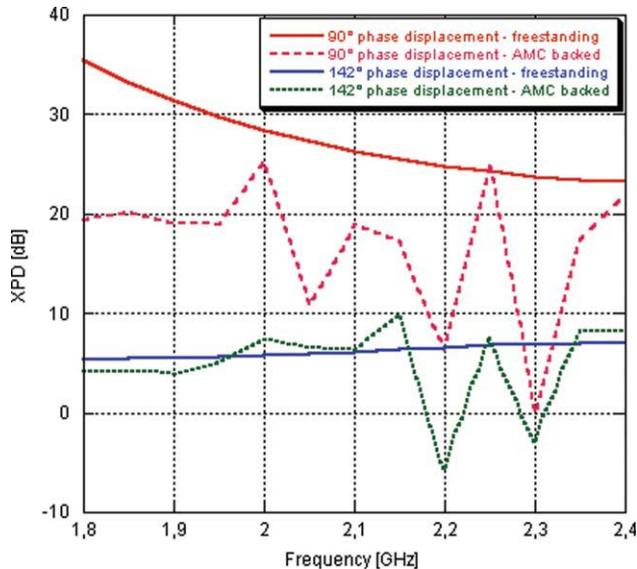
+90° phase displacement (perfect CP) and with a +142° phase displacement (EP), in freestanding configuration and in presence of the AMC screen. [Color figure can be viewed in the online issue, which is available at [www.interscience.wiley.com](http://www.interscience.wiley.com)]
