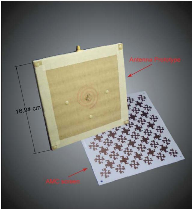
**Figure 1** Photograph of the realized AMC screen and antenna prototype. [Color figure can be viewed in the online issue, which is available at [www.interscience.wiley.com](http://www.interscience.wiley.com)]
