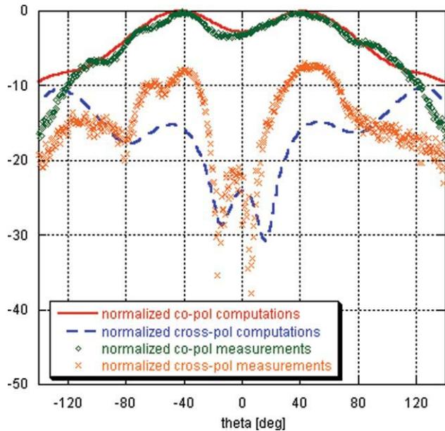
**Figure 6** Measured and computed radiation pattern (a) at 2.16 GHz in E plane ( $\varphi = 0^\circ$ ). [Color figure can be viewed in the online issue, which is available at [www.interscience.wiley.com](http://www.interscience.wiley.com)]
