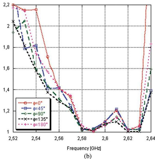
**Figure 5** (a) Axial ratio of the spiral closed to the AMC screen vs. azimuth angle for  $\theta = 0^\circ$ , in the first AMC band. (b) Axial ratio of the spiral closed to the AMC screen vs. azimuth angle for  $\theta = 0^\circ$ , in the second AMC band. [Color figure can be viewed in the online issue, which is available at [www.interscience.wiley.com](http://www.interscience.wiley.com)]
