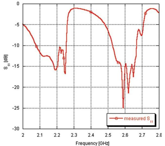
**Figure 8** Measured return loss of the spiral backed by the AMC. The antenna has been matched by using an ad hoc matching network. [Color figure can be viewed in the online issue, which is available at [www.interscience.wiley.com](http://www.interscience.wiley.com)]
