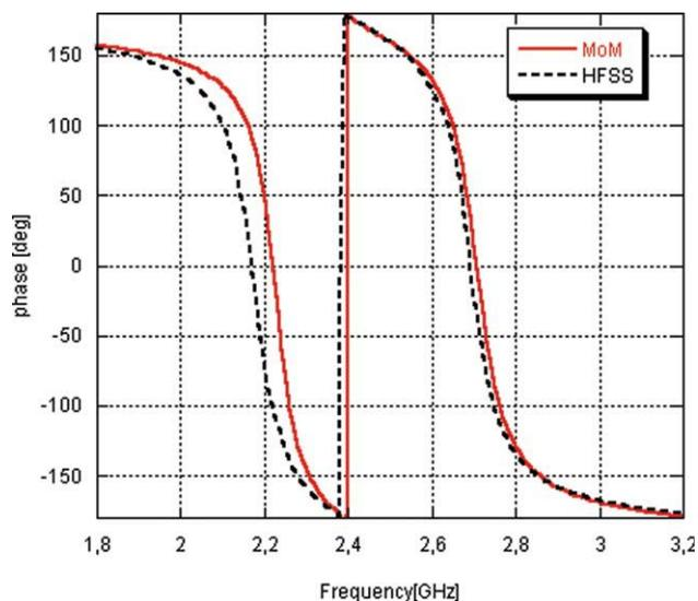
**Figure 2** Reflection coefficient phase of the AMC screen (MoM code results vs. HFSS results). [Color figure can be viewed in the online issue, which is available at [www.interscience.wiley.com](http://www.interscience.wiley.com)]
