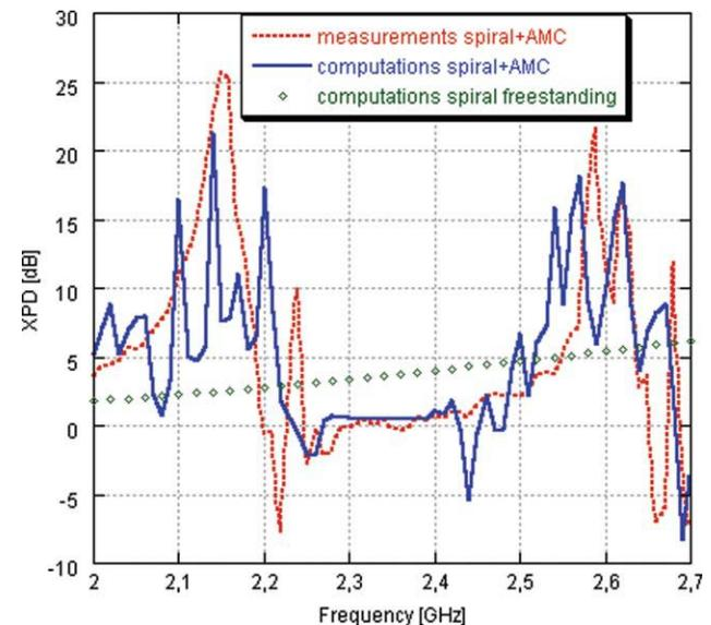
**Figure 3** Comparison between the cross polarization discrimination (measured and computed) of the AMC backed spiral and the freestanding spiral, in the boresight direction. [Color figure can be viewed in the online issue, which is available at [www.interscience.wiley.com](http://www.interscience.wiley.com)]
