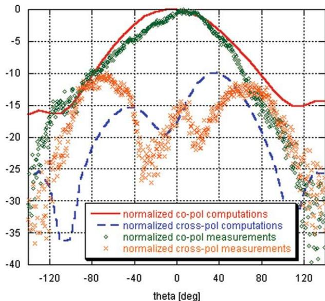
**Figure 7** Measured and computed radiation pattern (a) at 2.62 GHz in E plane ( $\varphi = 0^\circ$ ). [Color figure can be viewed in the online issue, which is available at [www.interscience.wiley.com](http://www.interscience.wiley.com)]
