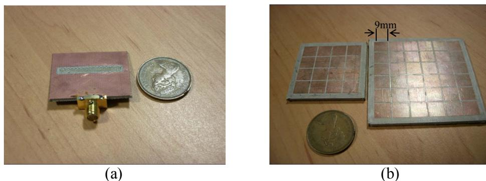
Fig. 1 (a) Slot antenna and (b) EBG structure (6 $\times$ 6 elements and 4 $\times$ 4 elements)
