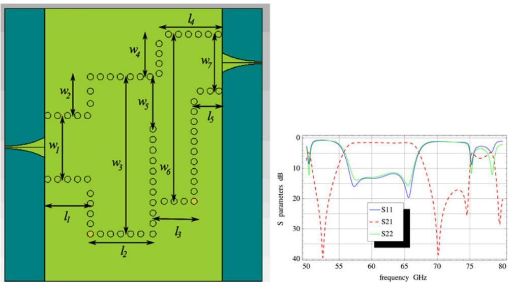
Fig. 8 Cavity filter design and simulated performance
