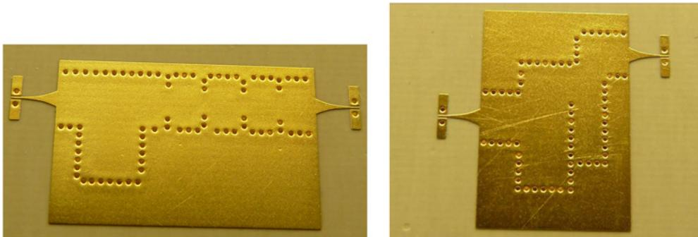
Fig. 11 *Manufactured filters*
