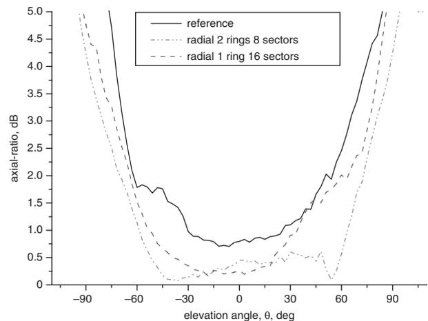
Fig. 3 Measured axial-ratio beamwidth at 1.575 GHz for three prototypes
