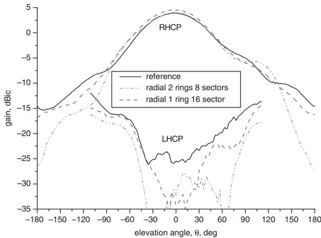
**Fig. 4** Measured RHCP and LHCP radiation pattern comparison at 1.575 GHz
