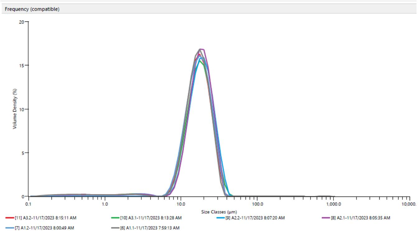
**Figure 5: Particle size analysis of glass bubbles used for BZ-1.**
