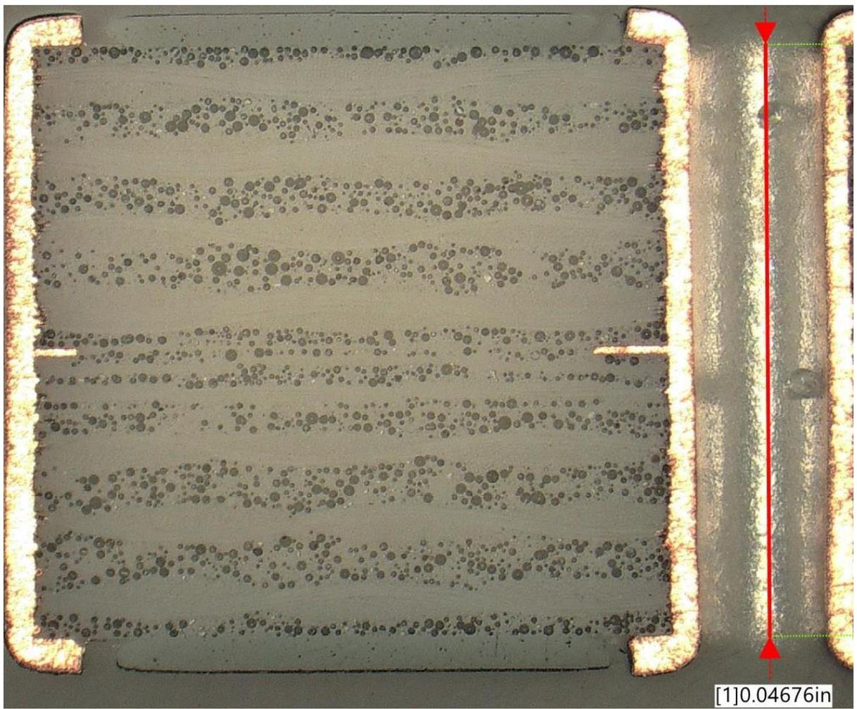
Figure 4: the cross-section of a multi-layer BZ-1 PCB; 100x magnification. At this scale, the presence of hollow glass spheres is easily observed.
