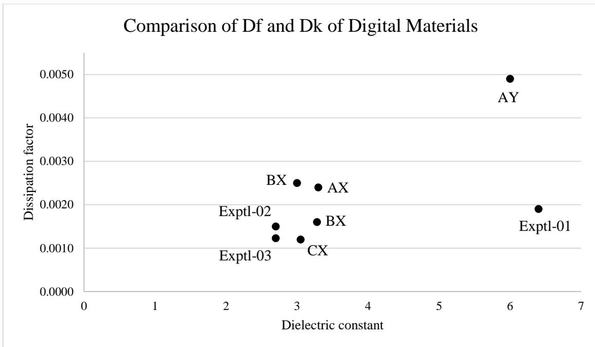
**Figure 3: The data from Table 1 is plotted to show the range of Dk and Df values achieved by changing the base resin and/or filler.**
