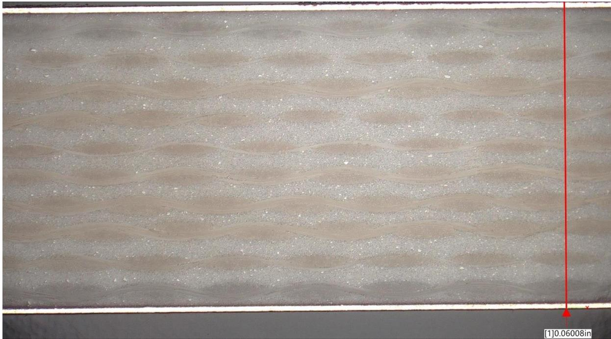
Figure 6: Cross-section of a 10-ply 2116SI dielectric CCL using hollow silica filler; 100x magnification.
