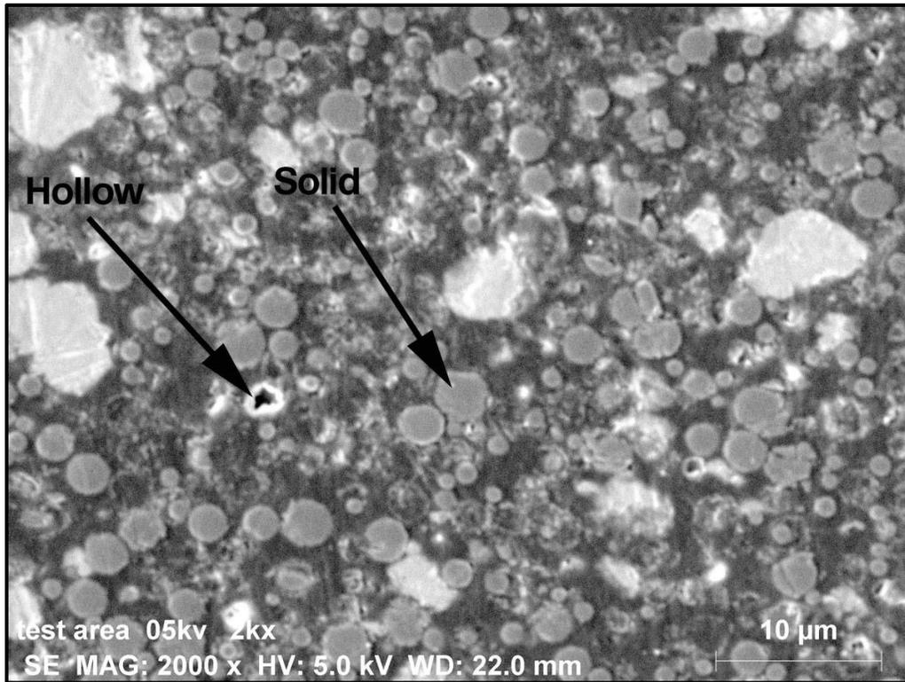
Figure 7: Cross-section of 10-ply 2116SI dielectric CCL using hollow silica filler; 2000x magnification. At this scale, it is possible to observe the spherical, hollow filler and some irregularly shaped pieces of insoluble materials.
