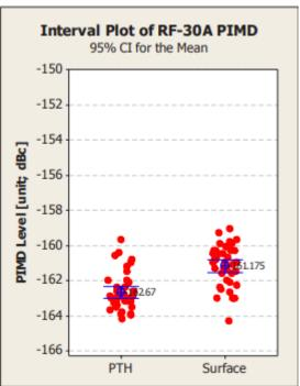
Condition; 20Watt(43dBm) source near 1800MHz, frequency sweep Test coupons; 50 Ohm microstripline with about 20 inch signal length
