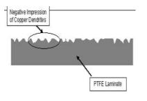
Figure 3 - Illustration of PTFE surface remaining after copper removal / etching
